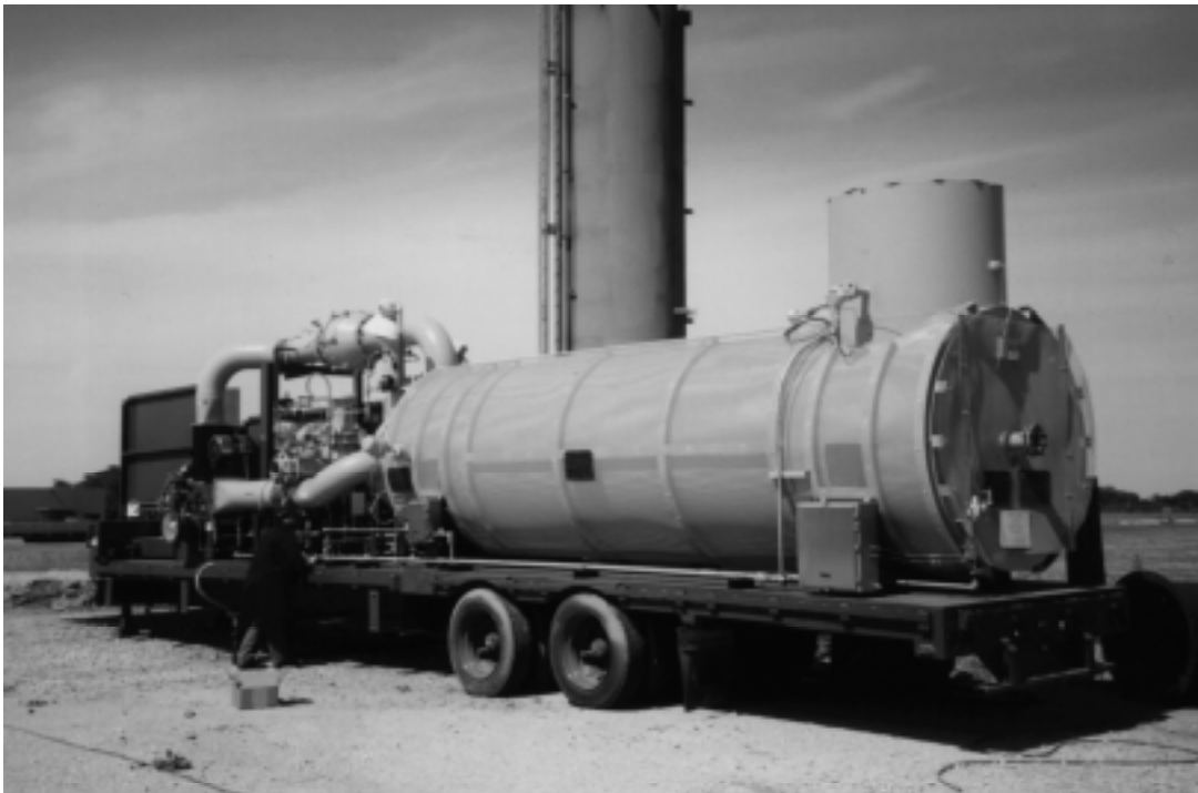
Figure 5-3—Example of Tank Mechanical Vapor-Freeing Equipment
